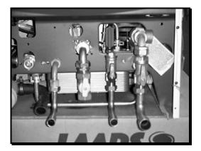
8. Connect and tighten part (k) <sup>3</sup>/<sub>4</sub> black handled ball valve to part (l) <sup>3</sup>/<sub>4</sub> x 90° copper elbow. Install assembly to (1) heating supply and tighten. Ensure all fittings are tight and aligned as shown.
