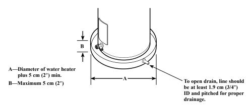
NOTICE: Auxiliary catch pan MUST conform to local codes. Catch Pan Kits are available from the store where the water heater was purchased, or any water heater distributor.
