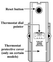
The illustration at the left shows the temperature adjustment dial used for setting the water temperature.
