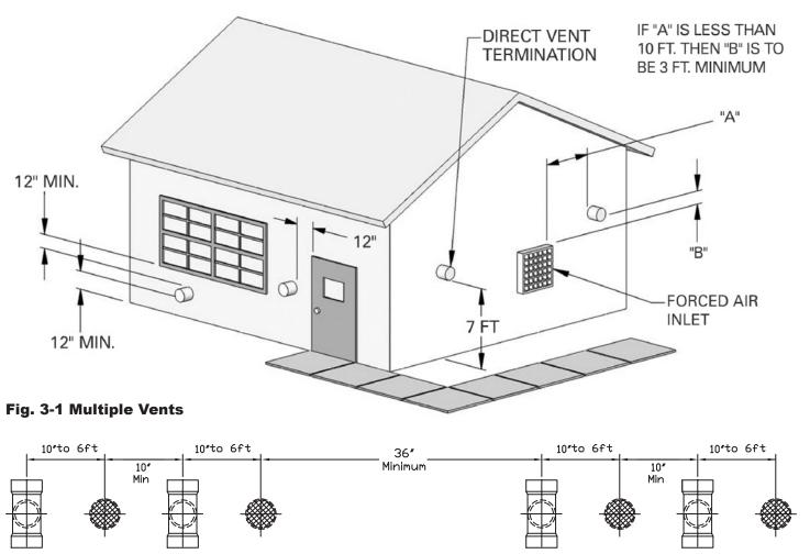
Fig. 3-2 Multiple Vent Spacing\*
