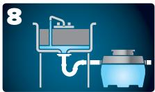
Make sure to run sinks to refill unit with cold water after pump-out.
