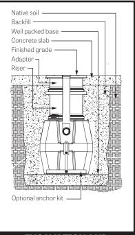
**EXCAVATION AND BACKFILL DETAIL**
