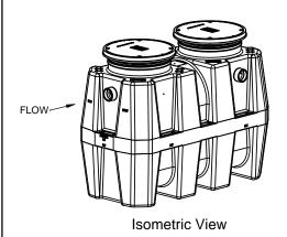
Set unit on level solid surface as close as possible to fixtures being served. If unit is to be installed below grade refer to below grade installation instructions. (sheet #3)
