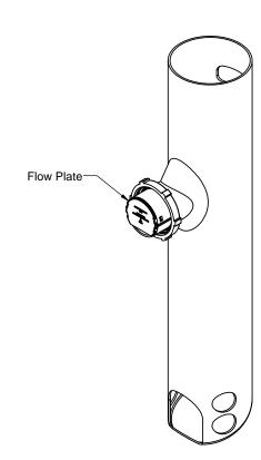
To maintain proper flow rate, when interceptor is installed in a high flow or increased head pressure application keep calibrated flow plate installed. Flow plate orifice calibrated to rated flow (GPM) at 13 foot water column.
