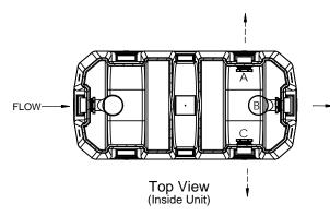
Connect outlet diffuser to the desired outlet (A,B,C). Unit is shipped with outlet diffuser in location B and sealing caps on locations A and C.
