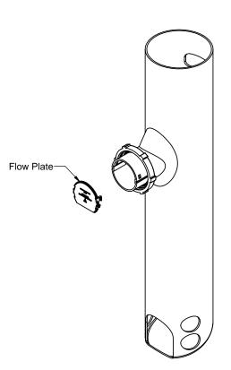
To maintain proper flow rate, when interceptor is installed in a low flow or reduced head pressure application remove and discard calibrated flow plate. Flow plate orifice calibrated to rated flow (GPM) at 13 foot water column
