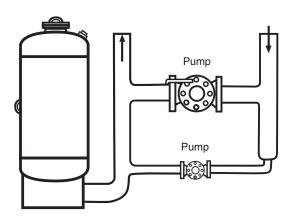
3. In a municipal well system or pressure boosting station, WELL-X-TROL®s are used to control sequential start of the main pumps. At the same time, it reduces surge and provides the jockey pump with guaranteed minimum run times during low peak demand periods.
