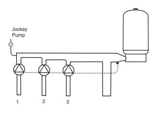
4. WELL-X-TROL® 400 Series are also used for high pressure booster applications, e.g. high rise buildings, irrigation systems and community wells.
