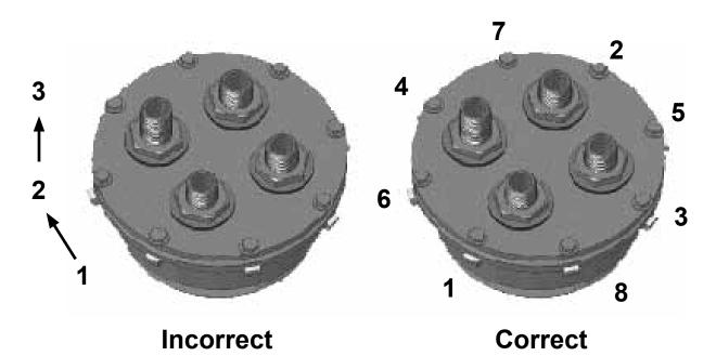
**CAUTION:** Does not require excessive force to seal properly.
