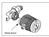
The Danfoss RAV operator is distinguished by the metal band connecting the operator to the valve.
