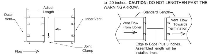
Step 3: Slide the Inner Vent into the Outer Vent to the desired overall length. Apply a 1/4" bead of RTV sealant completely around the vent at the joint. Smooth sealant into place.
