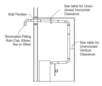
Unenclosed Vertical Vent and Horizontal Termination
