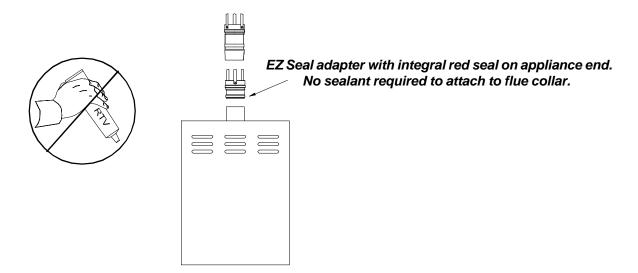
• If the integral red seal is only in the female end, you will need to use an approved hightemperature RTV silicone sealant to make the connection to the appliance. Follow the procedure recommended by the appliance manufacturer.
