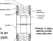
5. Secure the Wall Thimble to the interior sheathing using suitable fasteners.
