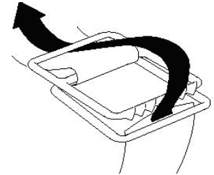
Figure 10 – Battery Hold-down Strap Threading
