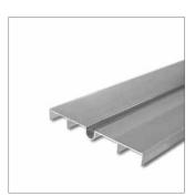
Furring strips are to be used in conjunction with 8 in. return bends to facilitate proper spacing of RAUPANEL and to provide a nailing surface for the floor covering. Reference the table below for product dimensions and square footage. Be sure to read the RAUPANEL System Installation Guide (855.625) for instructions on design and use of this product. RAUPANEL is 5/8 in. thick.
