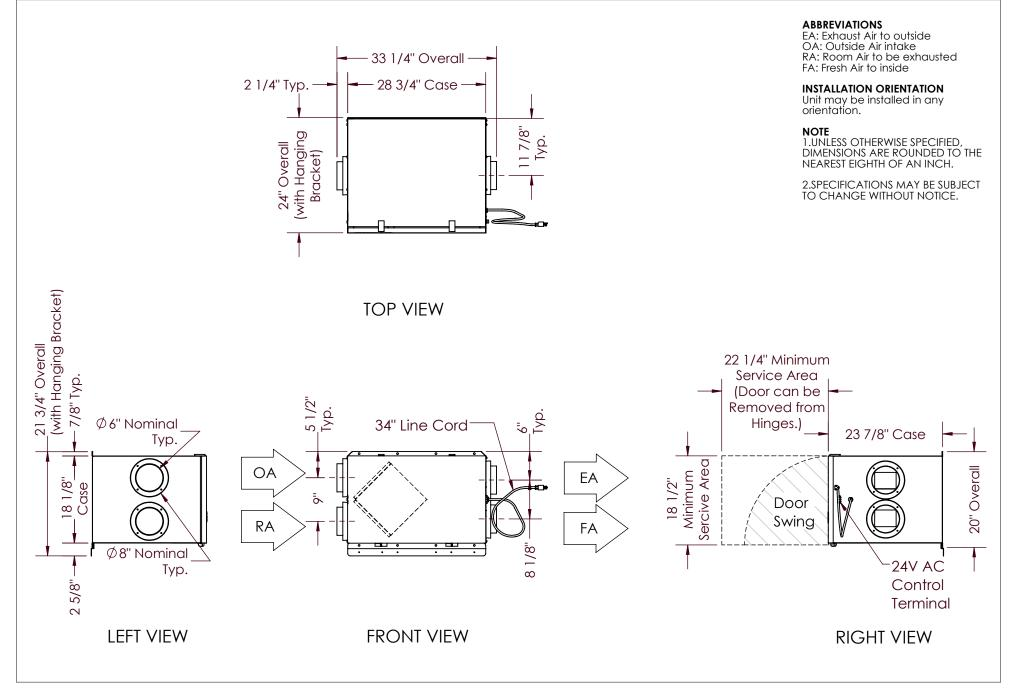
Model: EV200 Drawing Type: Unit Dimension Version: APR16
