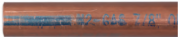
Figure 2 - Copper tube with "bad" surface scratch.
